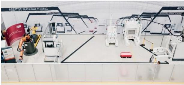
The built-up pilot plant of the NextGenAM project for automated additive manufacturing in detail, from left to right: band saw, Kuka robot, background: three-dimensional optical measurement system , setup station, unpacking station, forefront: automated guided vehicle (AGV), EOS M 400-4, not pictured: IPM M Powder Station L from EOS (Source: EOS).
