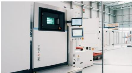
The additively manufactured parts are transported to the next process station under protective gas in a container on an automated guided vehicle. (Source: EOS).
