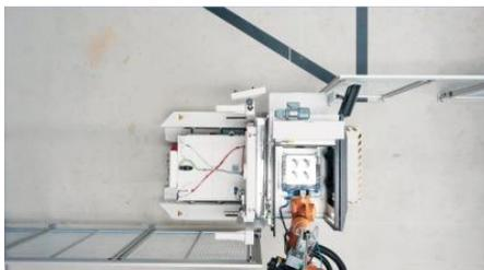
A robot removes the additively manufactured parts which are still on the build platform (Source: EOS).
