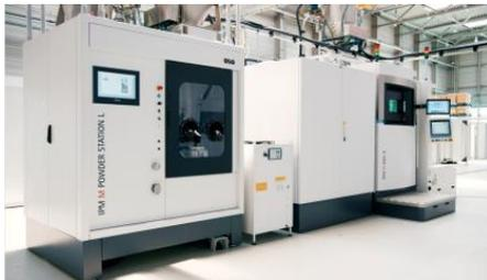
The IPM M Powder Station L feeds the EOS M 400-4 with powder material before and during building cycles and thus ensures sufficient powder at all times (Source: EOS).
