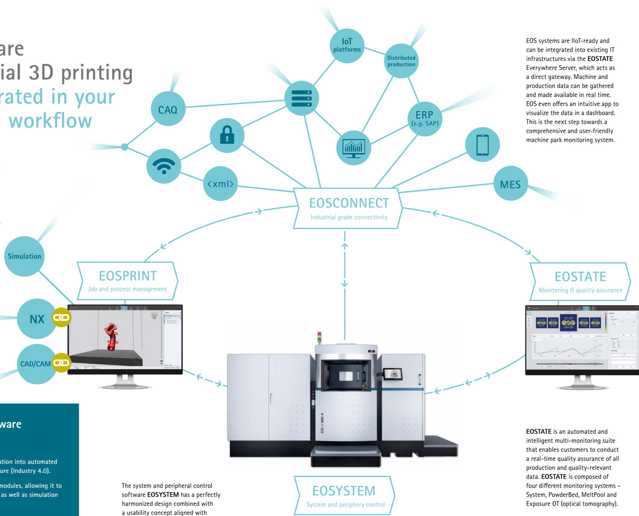
EOS systems are IIoT-ready and can be integrated into existing IT infrastructures via the **EOSTATE** Everywhere Server, which acts as a direct gateway. Machine and production data can be gathered and made available in real time. EOS even offers an intuitive app to visualize the data in a dashboard. This is the next step towards a comprehensive and user-friendly machine park monitoring system.
